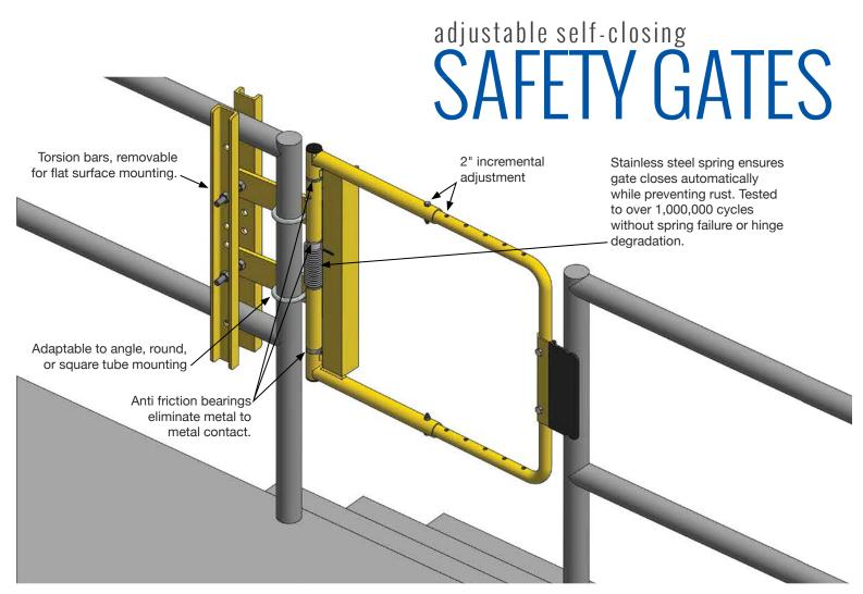
COTTERMAN<sup>®</sup> ADJUSTABLE SELF-CLOSING GATES can be used as barriers to prevent unintended egress through guardrail openings in accordance with OSHA and ANSI standards.
